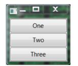
If we now send the window the resize message, the width of the frame is increased by a 100 pixels, but the buttons remain where they were *even though we had instructed the sizer to expand the buttons*.
